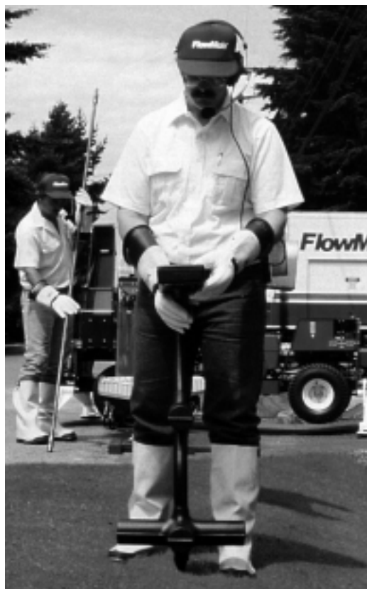
Figure 9. Field Gradient Tracking Receiver (FlowMole® FlowCator®)
