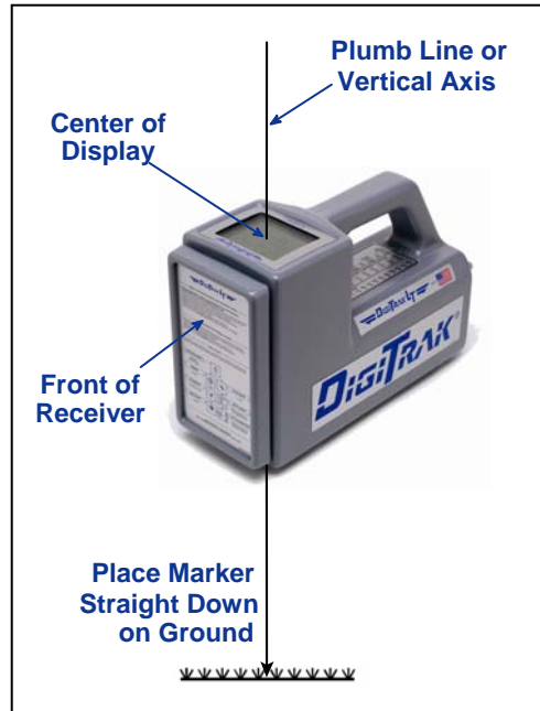
Plumb Line for Marking Locate Points
