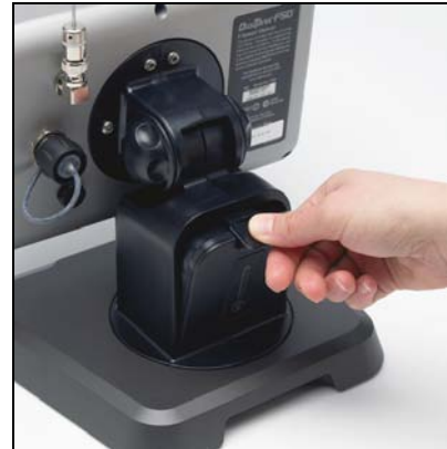
Installing FSD Battery
