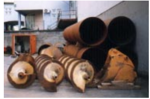
Auger sections and steel casings.
